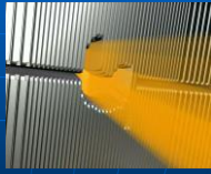
A multileaf collimator is used to shape the radiation beam to match the tumor, sparing surrounding healthy tissue
